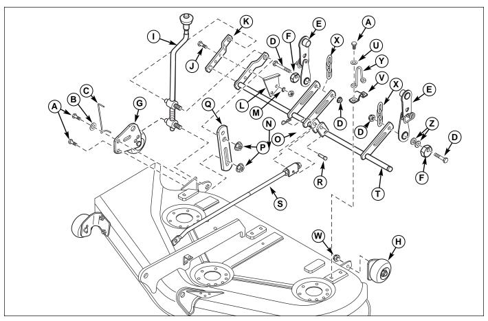
Figure 2. Remove Frame Hung Components
